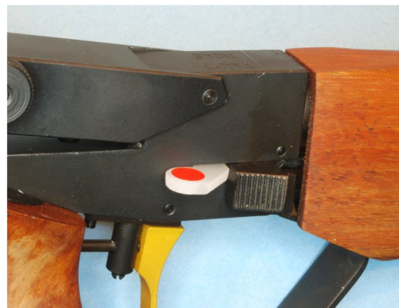
Figure 4: Dry fire adapter installed
